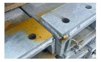
One is to provide a gap of at least 3/32-inch (2.5 mm) between the overlapped pieces using an intermittent fillet weld on all sides so that a pocket is not formed. This will ensure that all fluids drain out before galvanizing and that
