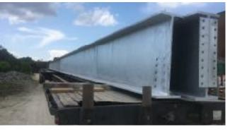
At Galvan, our large galvanizing kettle and our experience in "progressive dipping" techniques will allow almost any size fabrication to be galvanized. Here's a good example. We recently hot-dipped these massive beams: 75'1" in length, 33" tall, 11,500 lb. each. We handle it all, big and small. **Contact Galvan Industries today!**
